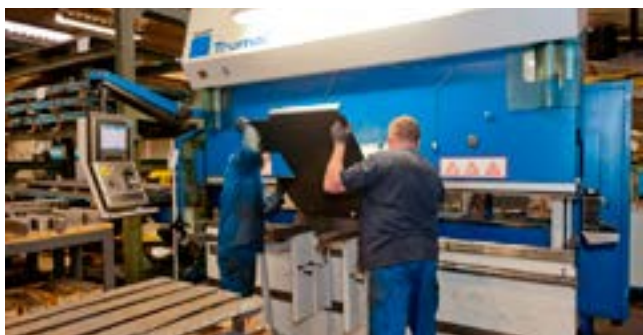
Computer assisted steel plate bending
